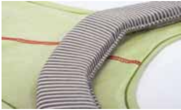
Breathable soft textile packaging of highly integrated electronics
